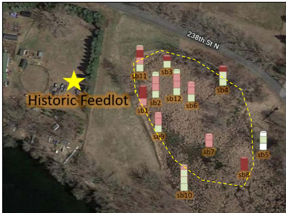
Figure 13. Plan view of the Bone Lake dairy wetland soil boring locations nearest to the past dairy feedlot with the soil boring phosphorus concentration results overlaid. The green colors indicate phosphorus levels in the normal ranges and the red or dark red colors indicate elevated levels. The yellow dashed line indicates the approximate area of the wetland that was excavated to remove the nutrient laden soils.
