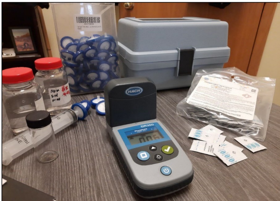
Figure 6. HACH Colorimeter and accessories used by the Comfort Lake–Forest Later Watershed District for their DIY sequential diagnostic assessment orthophosphate monitoring effort. Total cost for all equipment and supplies pictured was less than $700. After the initial investment in equipment, it costs less than $50 to analyze 100 water samples, or ~$0.50 per sample (not including staff time).
