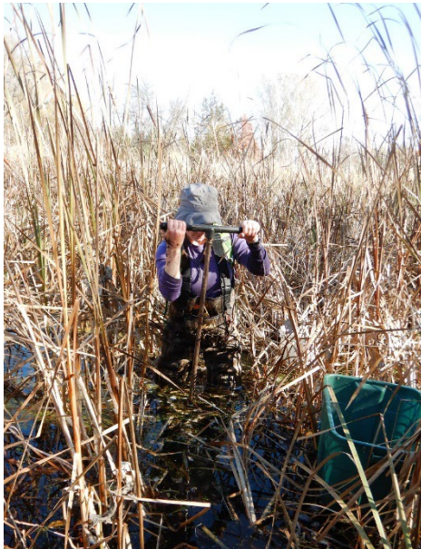
Figure 12. Soil borings being collected using a hand auger in the Bone Lake dairy wetland (left panel) and a representation of the soil samples collected (right panel).
