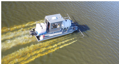
Left: Aerial photo of alum application barge on Shields Lake. The Shields Lake Alum Treatment reduced phosphorus loading to Forest Lake by an estimated 500 lbs/yr. Middle: Pre alum treatment on Moody Lake. Right: Post alum treatment on Moody Lake. The Moody Lake Alum Treatment reduced phosphorus loading to Bone Lake by an estimated 324 lbs/yr.
