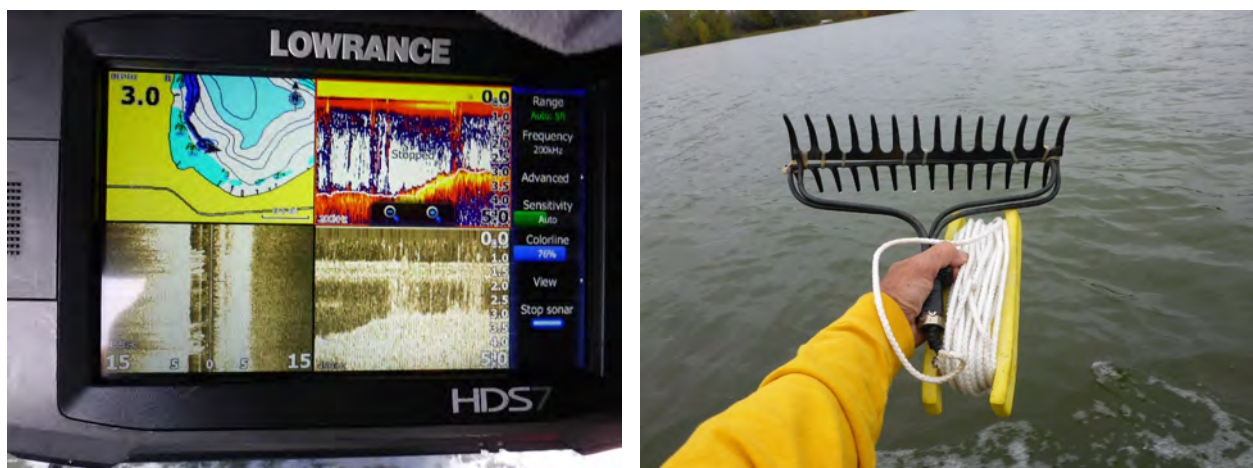
Figure 4. A high definition sonar (Lowrance HDS7) with downscan and sidescan features was used to identify potential submerged objects. A rake was dragged over the suspected obstacles to verify a potential snag.
