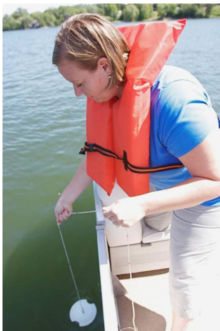
Measuring water clarity with Secchi Disc
