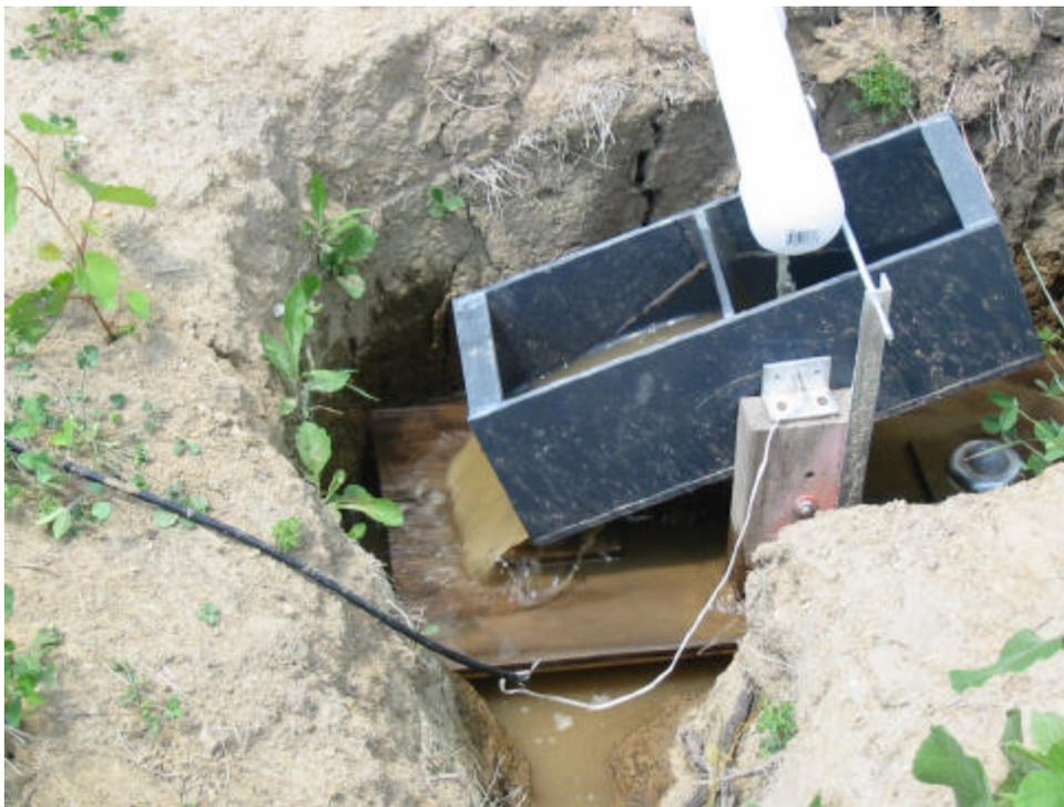
**Figure 6.** Tipping bucket runoff gauge during tip.
