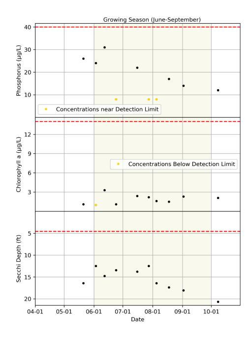
State standard are shown with a dashed red line. Phosphorus =  $40 \mu g/L$ , Chlorophyll-a =  $14 \mu g/L$ , Secchi Depth = 4.6 feet. Sample points are shown in black dots. Points above the line are worse than the State standard. Points below the line are better than the State standard.
