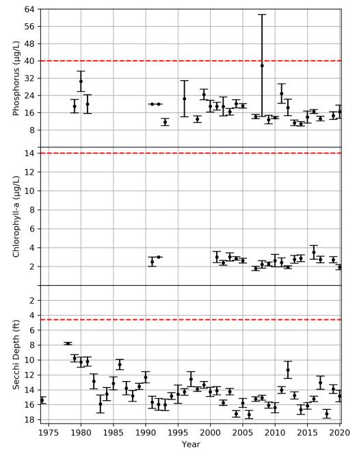
State standard are shown with a dashed red line: Phosphorus =  $40 \mu g/L$ , Chlorophyll-a =  $14 \mu g/L$ , Secchi Depth = 4.6 feet. Growing season averages are shown as black points. Points above the line are worse than the State standard. Points below the line are better than the State standard.
